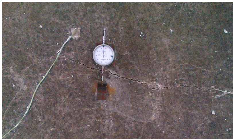
Figure 79. A thermal fracture during the SMRI test at Varangéville. The wall was cooled by \tau = -20^{\circ}\text{C} (Acknowledgements: G. Hévin, Storengy).
